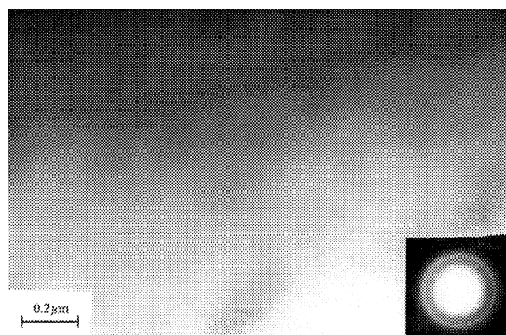
Fig. 3. The micro-structure of the boron film obtained by an transmission electron microscope at a position near an edge of a wedge-shaped boron film. The film is thicker toward top of the picture. The microstructure shows that the boron film is not porous. Insert at the bottom-right is its diffraction pattern. Absence of diffraction spots in the pattern indicates that the film is amorphous.
